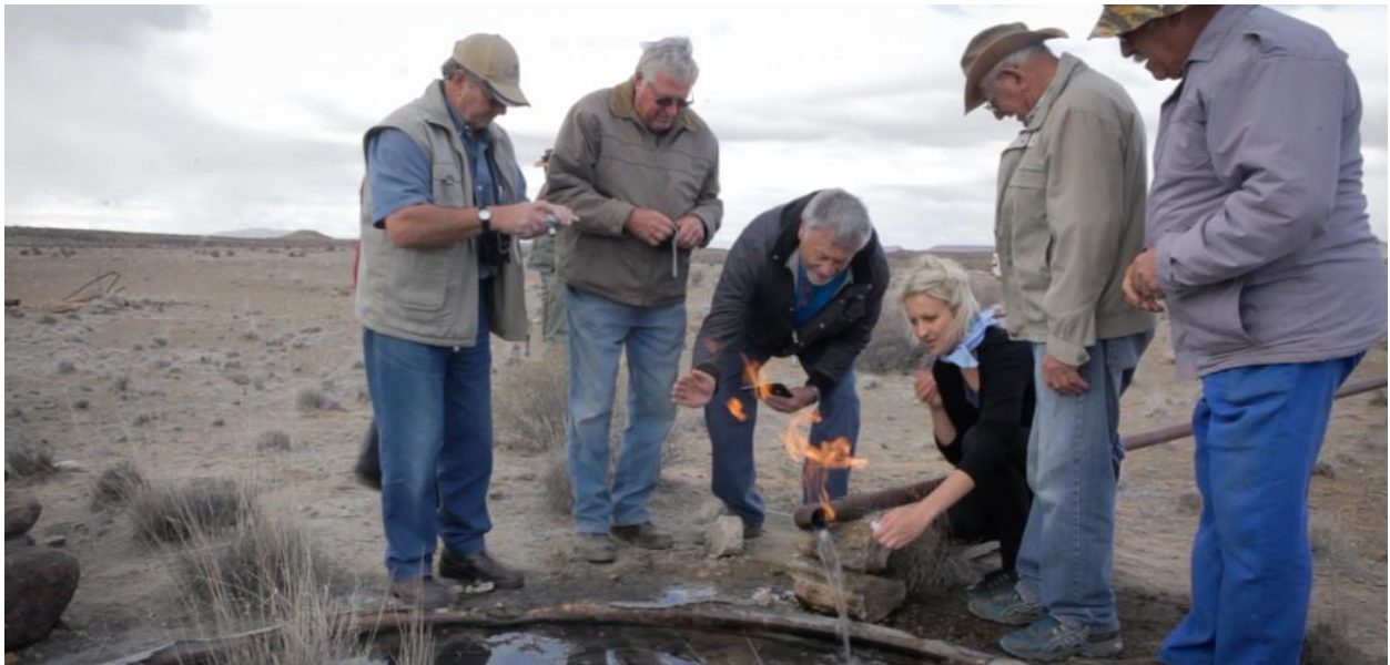
Figure 6.1: Tap leading from artesian borehole SA 1/66 drilled by Soekor. Warm water containing methane and a total dissolved salts value of 8,100 mg/l flowed from it once the tap was opened (van Tonder et al., 2013).
