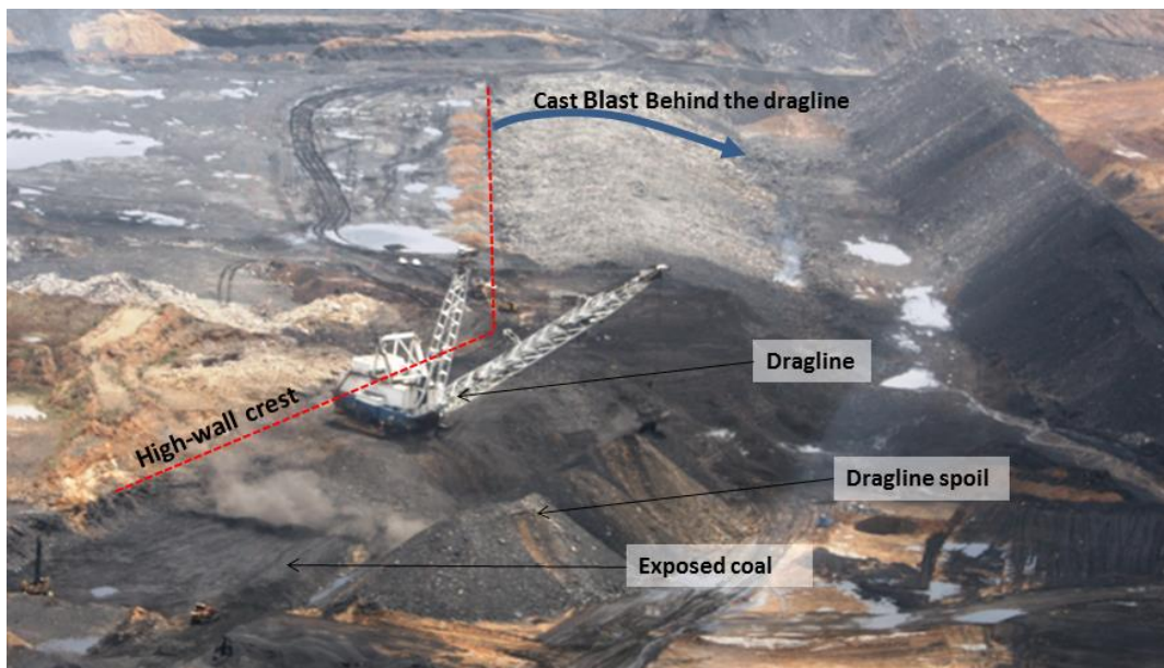
Figure 15: Photo of Interburden cast blast to be moved by dragline (Photo taken by Botha, 2013)
