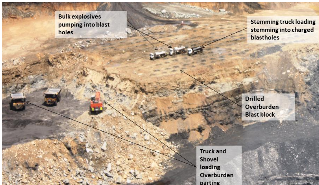
Figure 18: Photo of Overburden Blast preparation (Photo taken by Botha, 2013)
