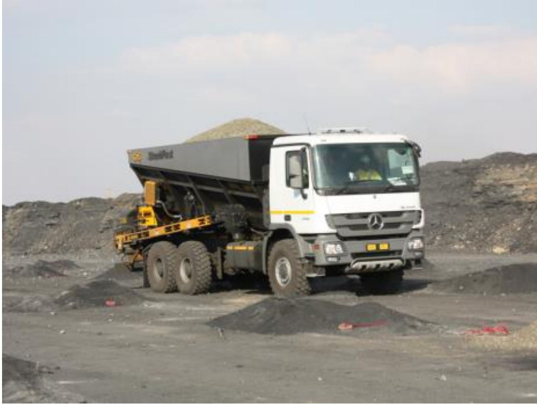
Figure 28: Stemming truck delivering crushed aggregate to the blast block (photograph taken by Botha, 2011)
