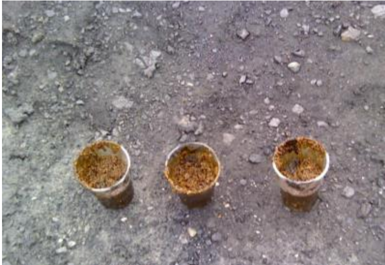
Figure 37: Cups filled with 250g explosive product for reactive testing (photograph taken by Botha, 2013)
