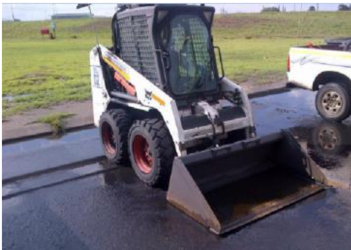
Figure 27: Photo of Skid Steer loader used for handling stemming material on a blast block
