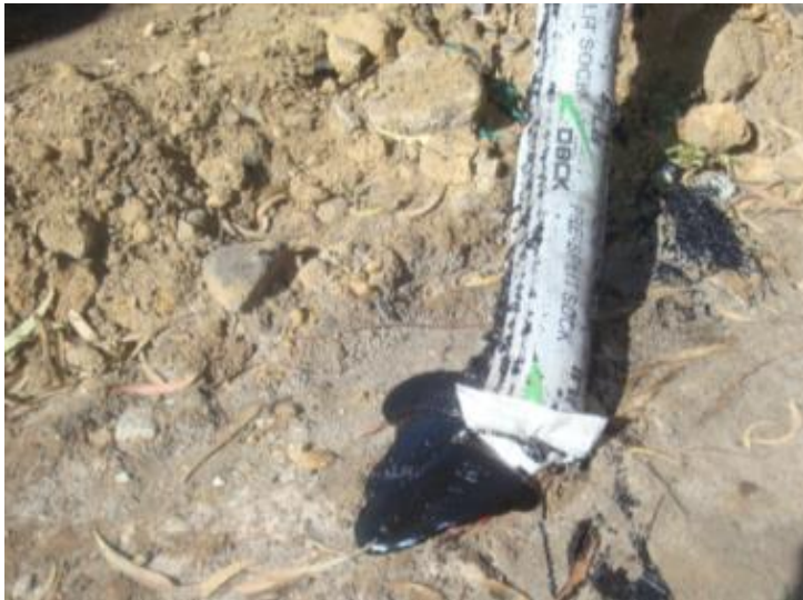
Figure 33: Close-up photo of suspended liners filled with explosives (Taken by Marton, 2011)
