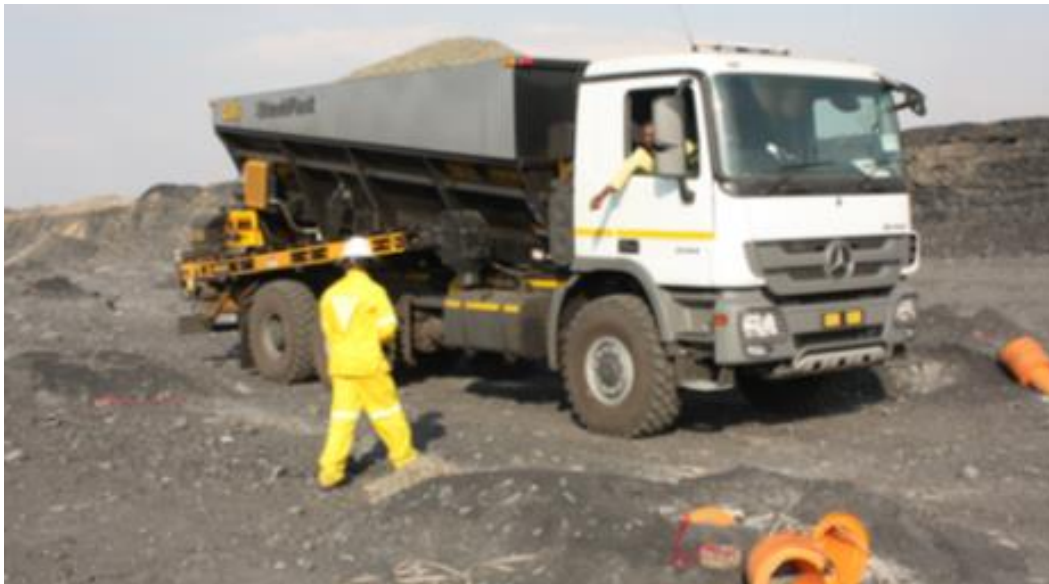
Figure 29: Stemming truck positioning on the blast block (photograph taken by Botha, 2011)
