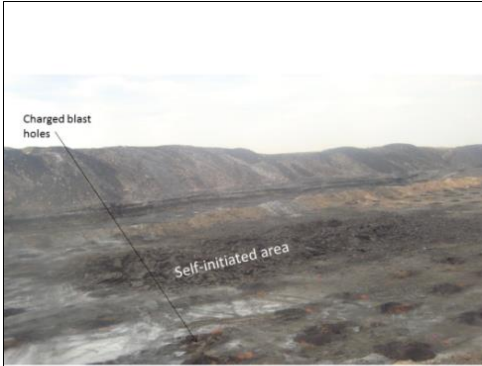
Figure 20: Photo of blast showing self-initiated area (Photo taken by Stenzel, 2010)
