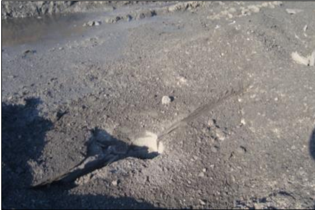
Figure 9: A pre-split hole after blast showing the split or crack formed (Photo taken by Botha, 2010)
