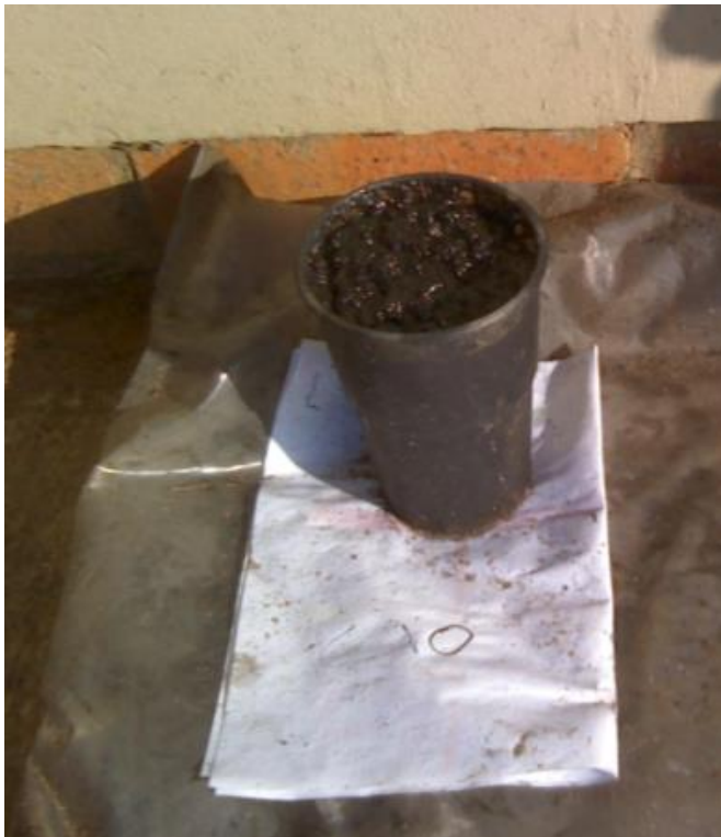
Figure 38: Test cup mix with drill chippings and emulsion explosives (photograph taken by Botha, 2013)
