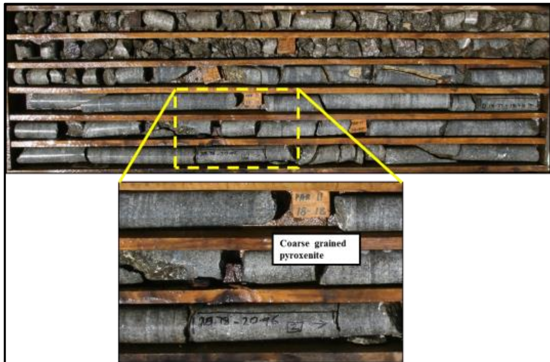
Fig. 3.2. Diamond drill core of the upper 16m weathered coarse grained pyroxenite of the PAR 11 borehole. More detailed insert shows micro-rhythmic layering (red arrows).
