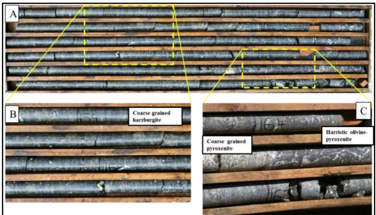
Fig. 3.4. Diamond drilled core from (A). 158.7 to 163.52m. (B) Typical coarse grained harzburgites. (C) Coarse feldspathic pyroxenite in contact with harristic-textured olivine-pyroxenite.
