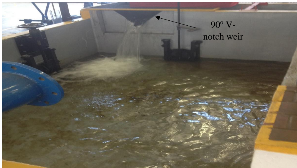
Figure 3.6 Tail-box terminating at a 90° V-notch weir (a tape measure glued to the wall of the tail-box was used to measure the depth of water)
