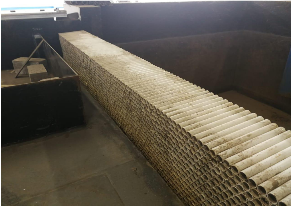
Figure 7.5 Honeycomb used to stabilise the flow-rate
