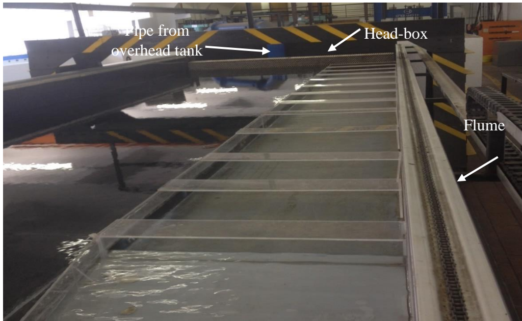
Figure 3.3 Upstream section of the constructed street model
