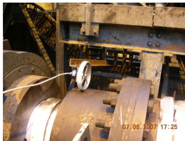
Figure 8 Speed Measurement by means of Tachometer
