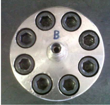
Figure 10: Top View of Pressure Vessel/Reactor B used in the adsorption capacity testing
