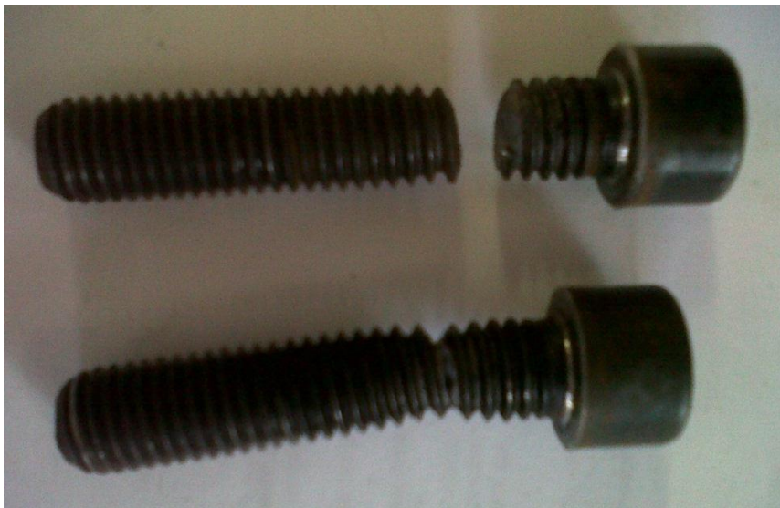
Figure 27: Sheared and snapped bolt from the pressure vessels/reactors
