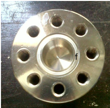
Figure 11: Internal view of the pressure vessel/reactor used to hold the coal samples
