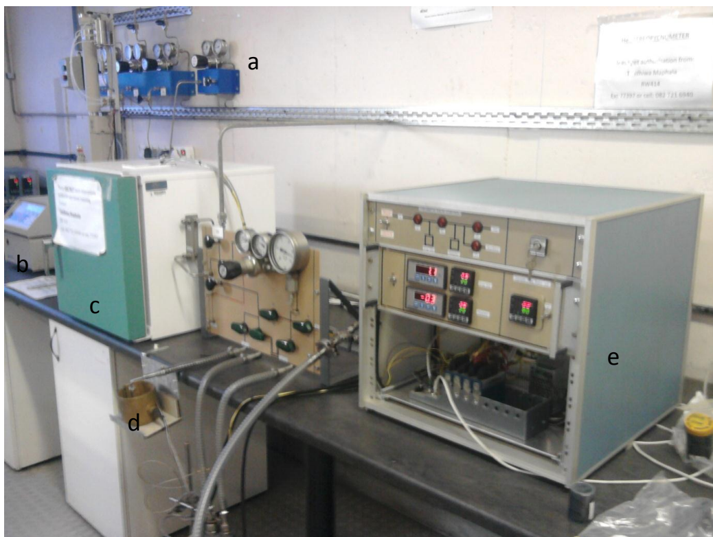
Figure 9: Picture of the laboratory adsorption equipment showing the pump, oven, degassing system, and the data logging system (see text for annotations)
