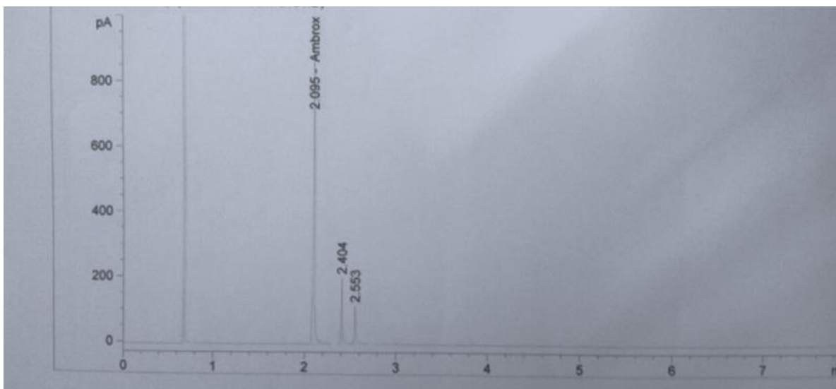
Figure 43: (-) Ambrafuran peak produced in a reaction without \text{MgSO}_2 anhydrous by zeolite CFG-1
