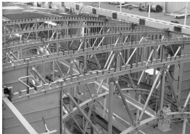
Figure 1.2 Mid-fuselage structure of Space Shuttle Orbiter showing boron-aluminum tubes [2].
