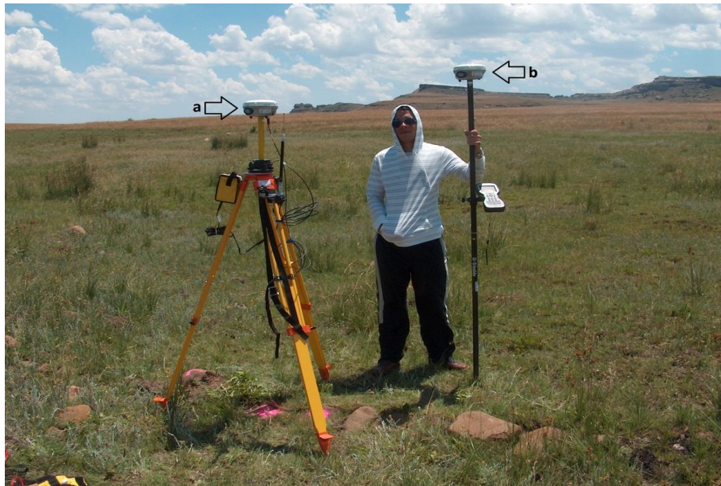
Figure 30: (a) DGPS base station and (b) rover.
