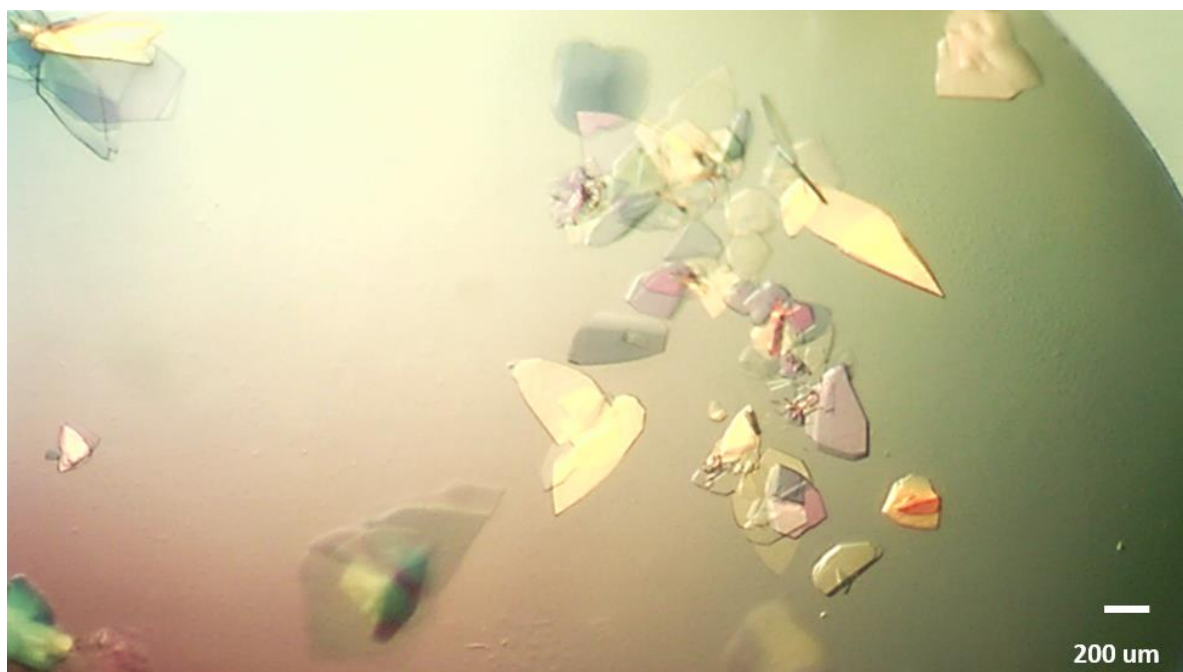
Figure 26. A bouquet of plate-like protein-DNA crystals obtained by vapor diffusion rate control. Crystal trials of the TBR1 T-box domain in the presence of SSL DNA were performed at 20 °C by using 0.5 mM SSL DNA duplex and 0.42 mM TBR1 T-box domain. A bouquet of very thin plate-like crystals appeared after 1 week in sitting drops containing 1.5 \mu L of DNA/protein solution and 1.5 \mu L of crystal solution 3 (100 mM 4-morpholineethanesulfonic acid pH 6.5, 200 mM MgCl_2 and 25% (w/v) PEG 4 000), equilibrated against 250 \mu L of crystal solution 3, overlaid with 50 \mu L of Al's oil (50% (v/v) paraffin oil and 50% (v/v) silicon oil). The crystals were harvested with a CrystalCap SPINE HT goniometer base fitted with either a 0.2 – 0.3 mm, 0.3 – 0.4 mm or 0.4 – 0.5 mm Mounted CryoLoop™ (Hampton Research, USA). The crystals were then cryoprotected by 3 dips in either 100 (v/v) Parabar (Hampton Research, USA), 30% (v/v) glycerol (made up with mother liquor) or 30% PEG (made up with mother liquor) and frozen in liquid nitrogen. Data collection was unsuccessful as the crystals were just too thin to cause significant diffraction.
