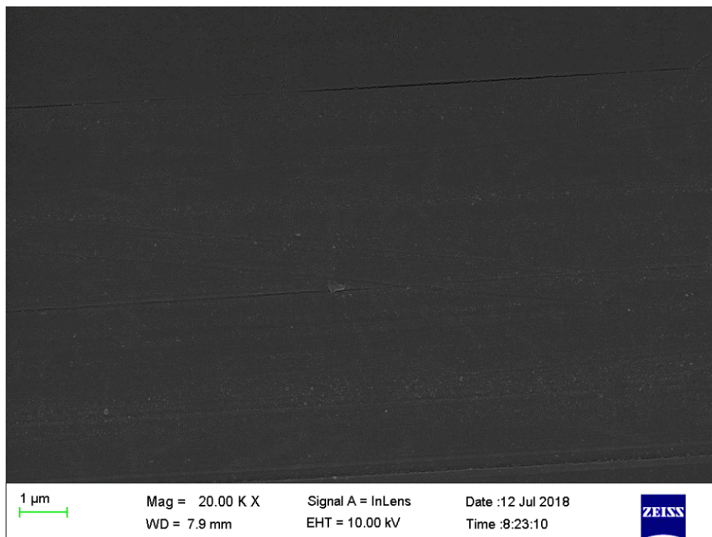
Figure 5.8 SEM image of the control PIM, PIM 0 (100% PSF)
