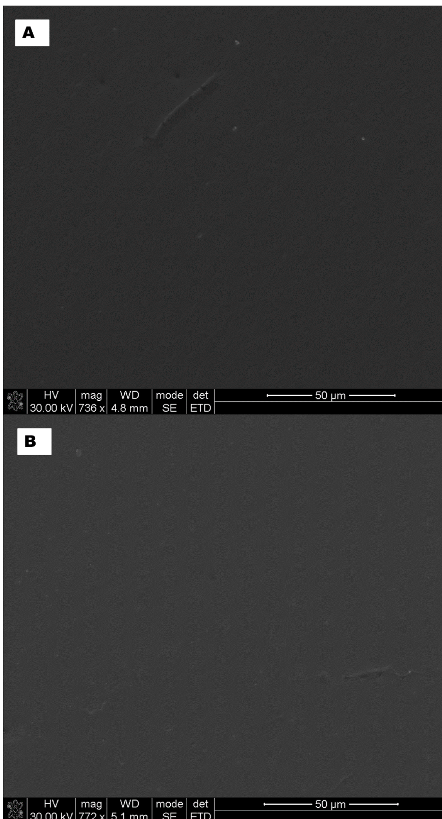
Figure 5.2 SEM images of solvent evaporation prepared PIMs at different composition ratios. A = 60:30:10 and B = 40:40:20
