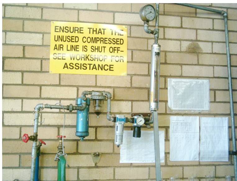
Figure 3B: The equipment used to control gas flow rate to the water-kerosene bath.
