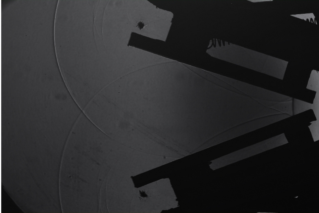
Figure 8.49: Shadowgraph of copper vs. glass (reversed) at 70^\circ and M1.3835
