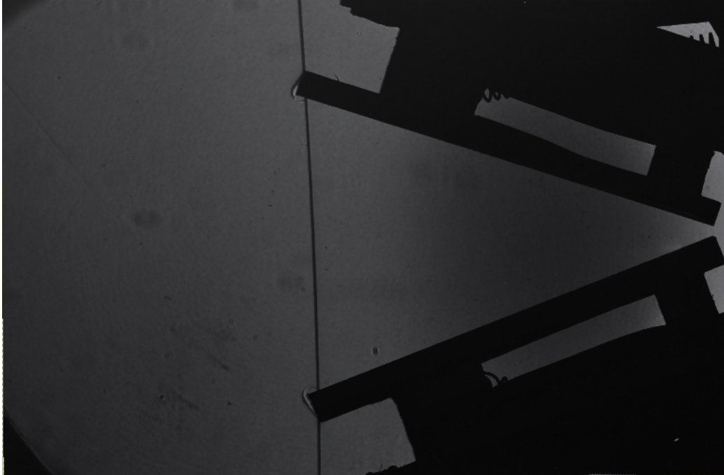
Figure 8.51: Shadowgraph of glass vs. copper at 70^\circ and M1.3058
