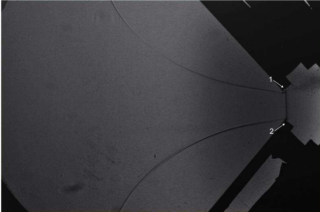
Figure 8.24: Shadowgraph of brass vs. aluminium at 40^\circ and M1.3888
