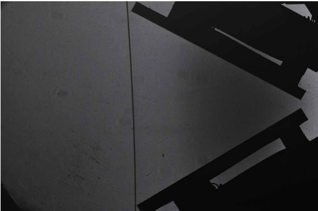
Figure 8.53: Shadowgraph of glass vs. copper at 60° and M1.3053
