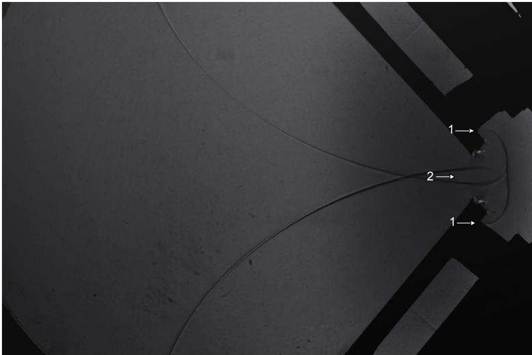
Figure 8.21: Shadowgraph of steel vs. steel at 40^\circ and M1.3519
