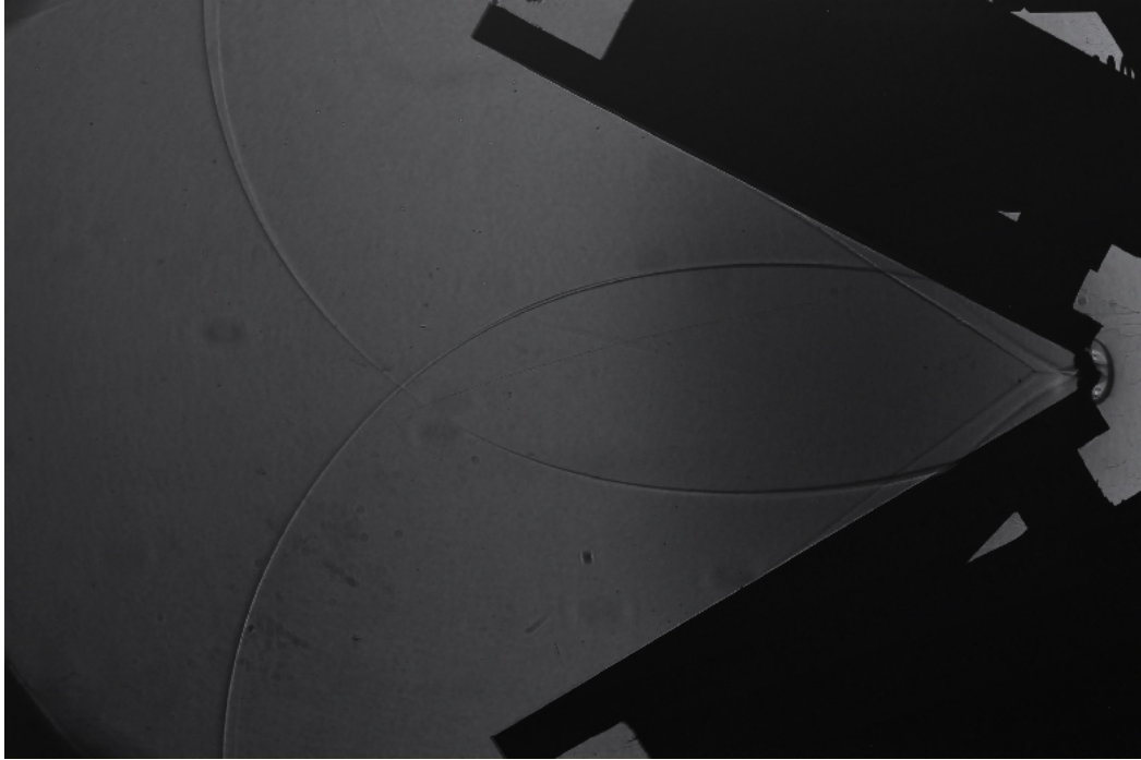
Figure 8.48: Shadowgraph of glass vs. copper at 60^\circ and M1.3974
