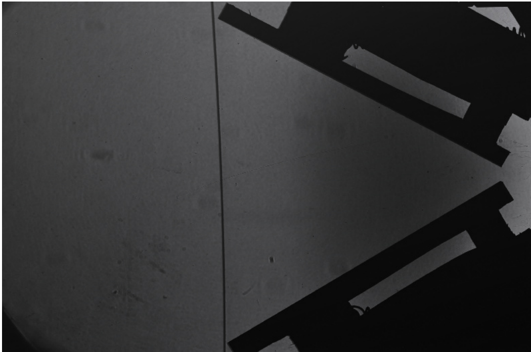
Figure 8.52: Shadowgraph of glass vs. copper at 60° and M1.3062
