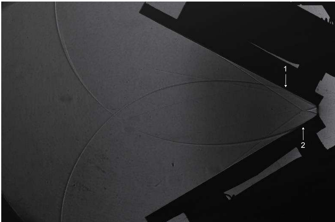
Figure 8.47: Shadowgraph of glass vs. copper at 60^\circ and M1.3534
