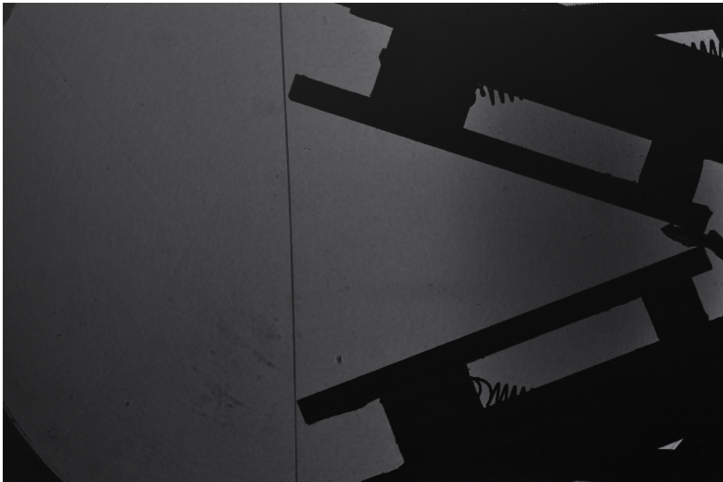
Figure 8.50: Shadowgraph of steel vs. steel at 70^\circ and M1.3883
