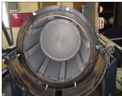
Figure 3.2 Picture of the laboratory grinding mill used for the experiments.
