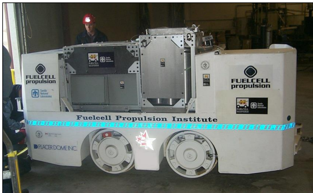
Figure 2.10: Fuel cell locomotive used in an underground gold mine in 2002 (Miller, et al., 2012)
