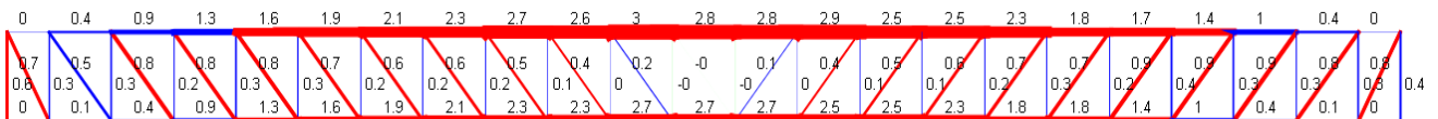
Figure 2.8: The VWO method solution of the truss frame showing the deflection contribution of each member (in mm) to the overall vertical deflection of the critical node. The members are not grouped. Line thickness represents magnitude of deflection. Red members are sized based on deflection consideration; Green members have a negative contribution to the overall deflection and are sized based on strength; Blue members are controlled by strength criteria.
