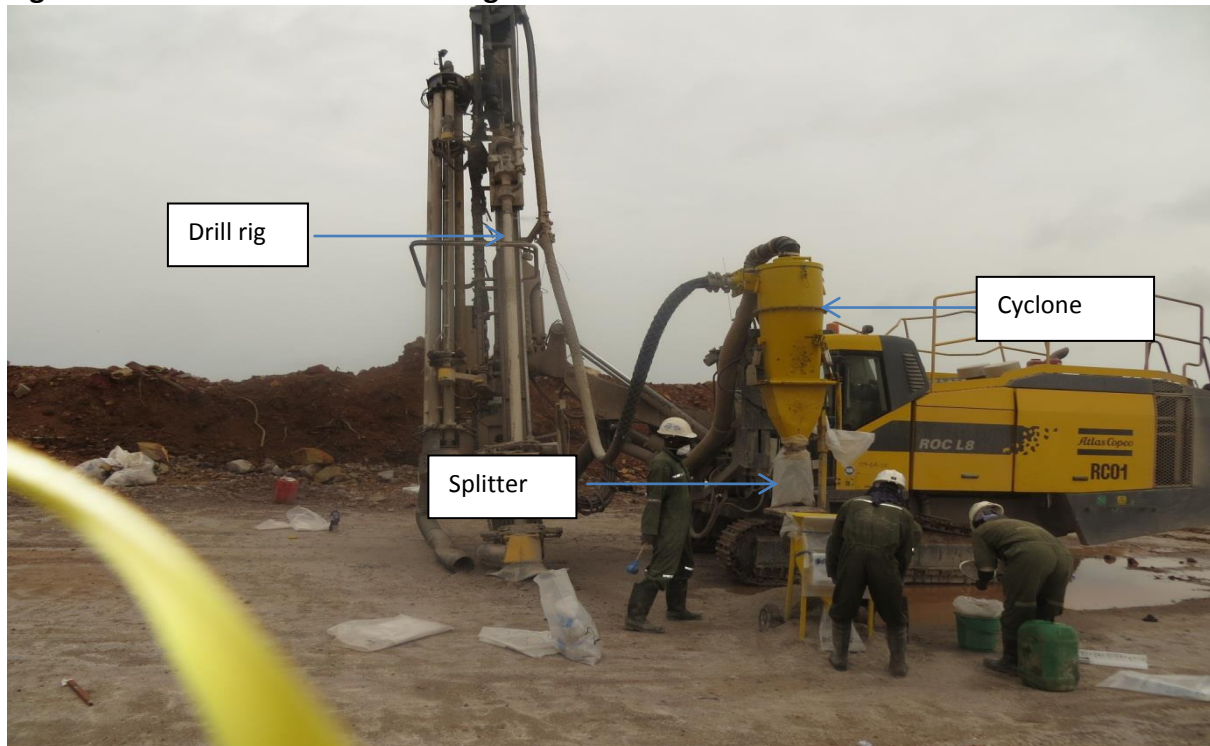
Figure 3.6 Reverse circulation drill rig
