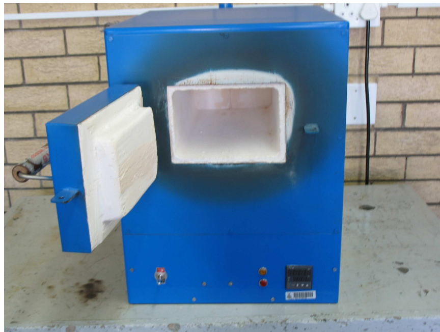
Figure 3.1: Furnace used for heat treatment.
