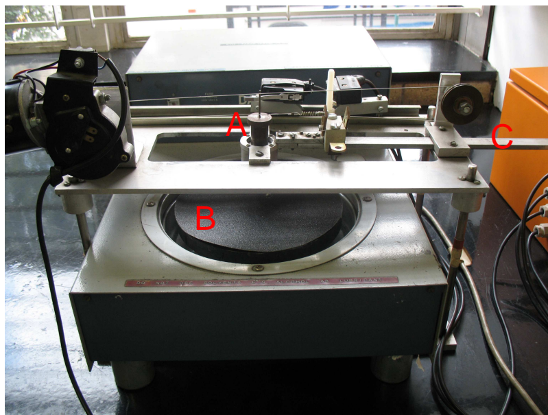
Figure 3.4: Photograph of the 2-body sliding wear apparatus, A is the sample holder, B is the SiC abrasive paper, C is the loading arm.
