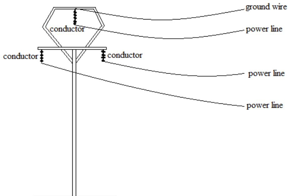
*Figure 1.4:* A diagram of a typical kite structure with a ground wire, three lines, and three conductors.
