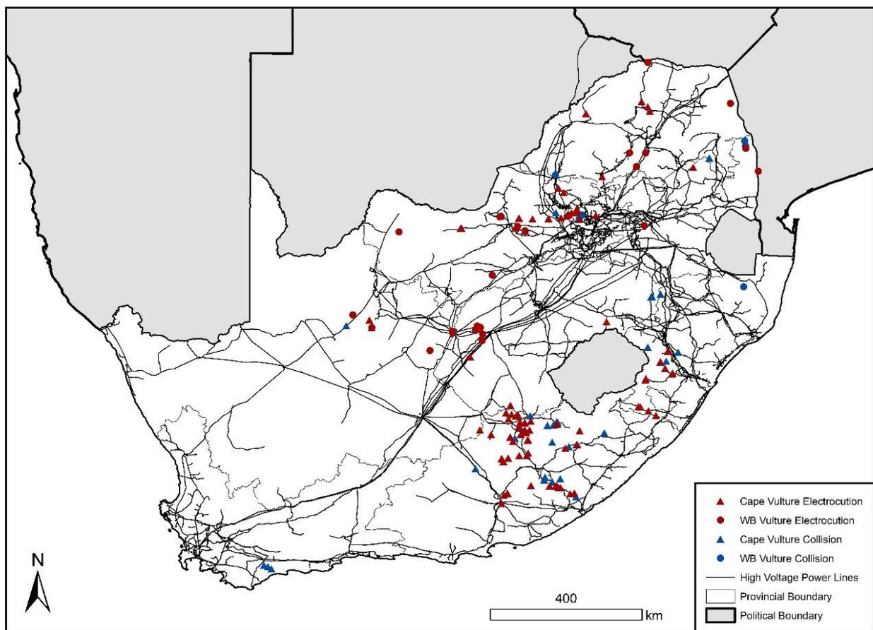
Figure 4.2: A map illustrating all major power lines in South Africa with all power line mortality points (collision and electrocution) marked.
