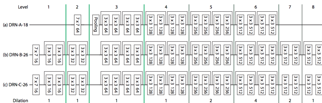
Figure 2.7: Three DRN architectures are shown above, namely DRN-A, DRN-B and DRN-C. DRN-C effectively reduces “gridding” artifacts that are introduced during dilation [Yu et al. 2017].
