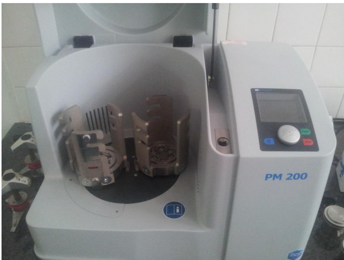
Figure 2.2 Planetary ball mill used for mechanochemical synthesis.
