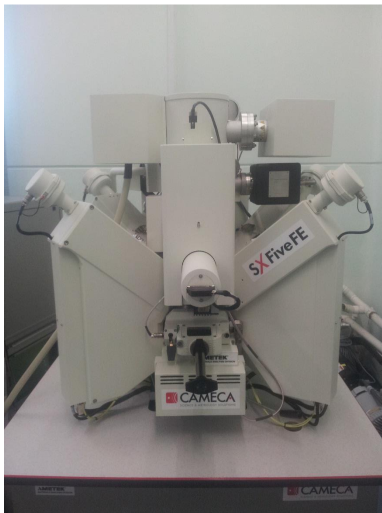
Figure 2.7: The CAMECA SX-5-FE Electron Probe Micro-Analyzer
