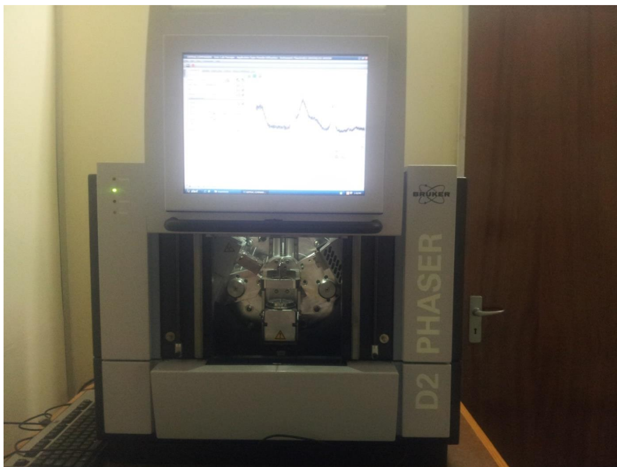
Figure 2.5: Bruker D2 phaser diffractometer equipped with cobalt radiation
