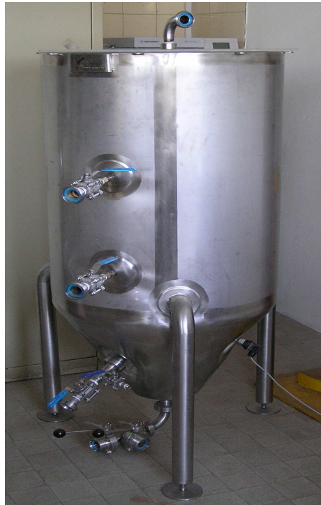
Fig 2.6. Conical Fermentation Tank (100L) of the Wits Microbrewery Plant.
