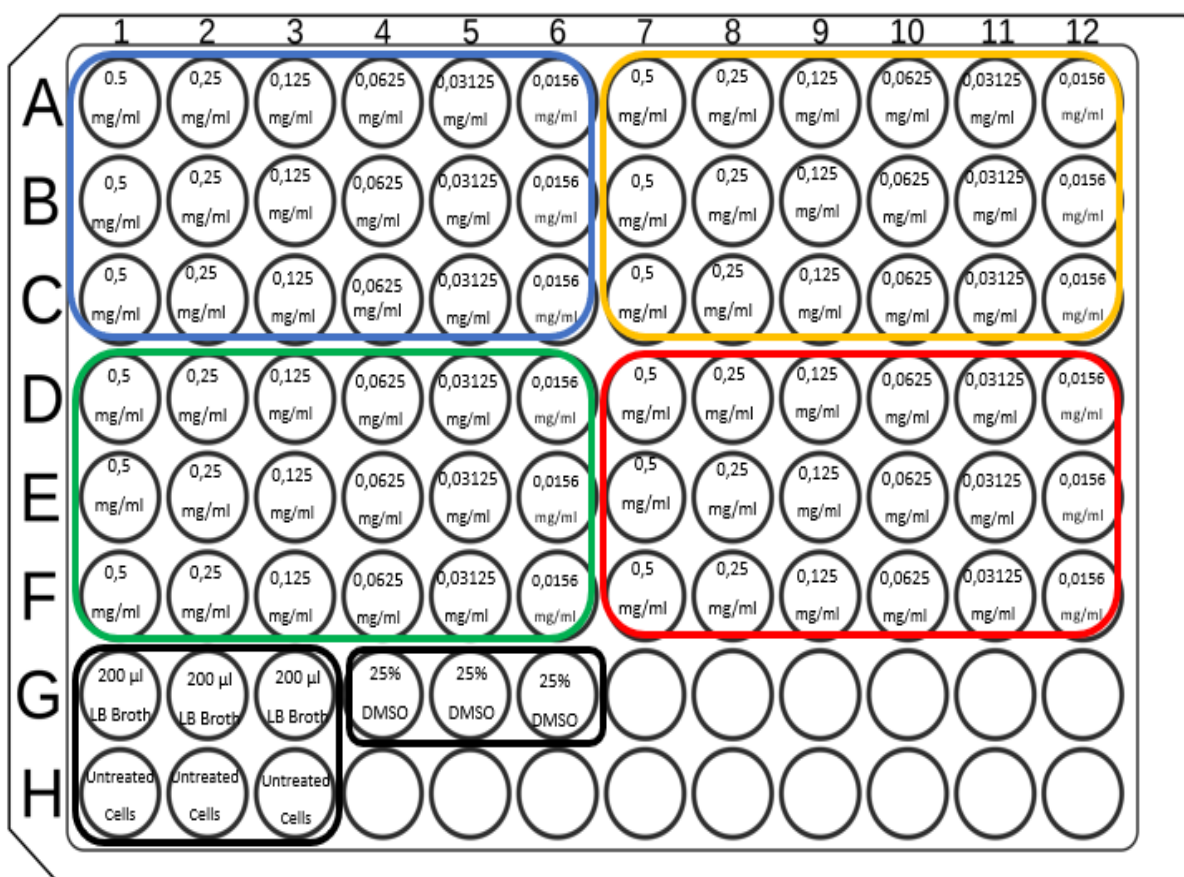
Figure 2.1: Template illustrating how the 96-well plates were prepared and the concentration range used for minimum inhibitory concentration studies for the broth dilution method. Serial dilutions of the compounds (silver(I) or positive controls silver nitrate and silver sulfadiazine) were done on the Enterobacter xiangfangensis pathogens. In addition, a positive untreated, negative media control and vehicle control, 25% (w/v) DMSO was also included. A total of eight different silver (I) phosphine compounds were tested, and 4 compounds were serially diluted in one plate (the colours on the plate indicate different treatments: UJ1, UJ2, UJ3, UJ4).
