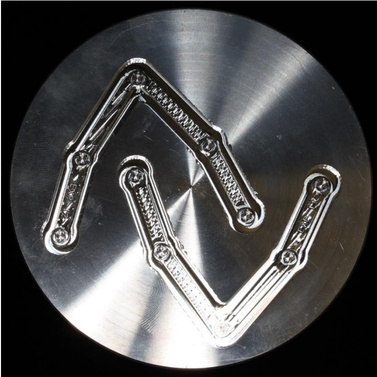
Figure 3.14 Milled frameworks in aluminium blanks (ASTM B348, Acnis, Villeurbanne, France)
