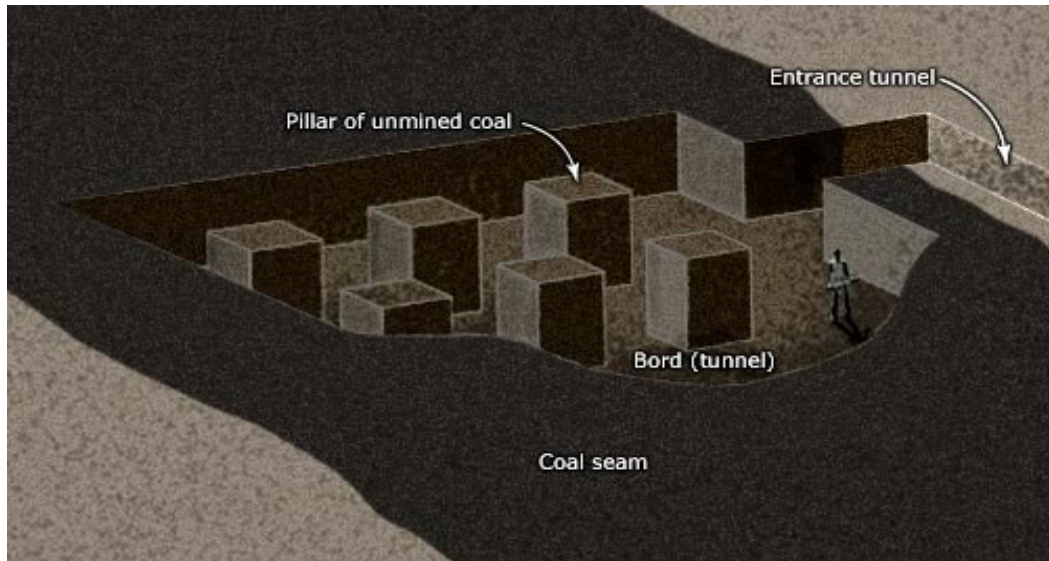
Figure 2-1: Bord and pillar mining technique (Alan and Jock, 2016)
