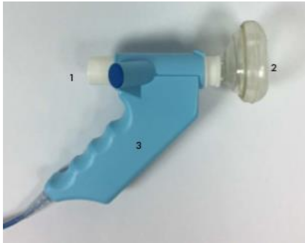
Figure 2.8: Equipment for the measurement of lung function with the EXHALYSER D during TBFVL and MBW measurements (1. Dead space reducer, 2. Face mask, 3. Flow head) (Used with permission: Mr Dirk Wendt, CEO ECO MEDICS AG (Duernten, Switzerland)).
