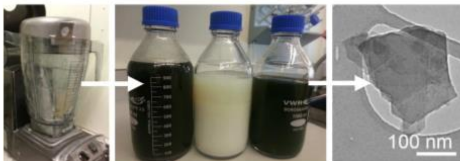
Figure 5: Using shear force from a blender to exfoliate bulk TMD crystals. 21
