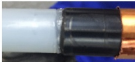
Figure 3.4: XLPE Ring Cut Defect
