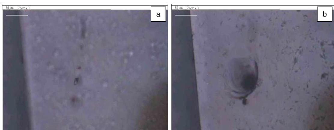
Figure 8.5. (a) Reflected light image of secondary aqueo-carbonic trail inclusions hosted in quartz of the Chambishi samples prior to laser ablation, and (b) post laser ablation. Flinc. no. CBSqz3By(4)11.
