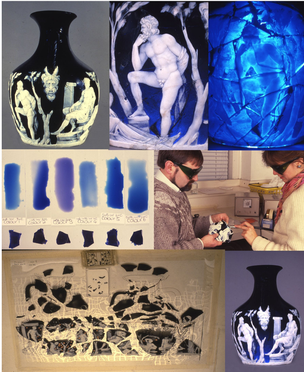
9. Collage picture showing the restoration of the Portland Vase (from top left to bottom right): the vase before dismantled for repair; detail in natural light; the break lines and filled areas were emphasized by flooding the inside of the vase with an intense ultraviolet light – the individual shards of glass could then be identified; resin fill tests (to replace gaps between shards after repair); conservators using UV setting adhesive to join the fragments; vase in fragments laid out ready for reconstruction on a plan; the vase after restoration is complete. © Trustees of the British Museum
