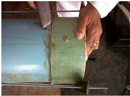
c) The use of knife to remove silicon sealer at the conjunctions
