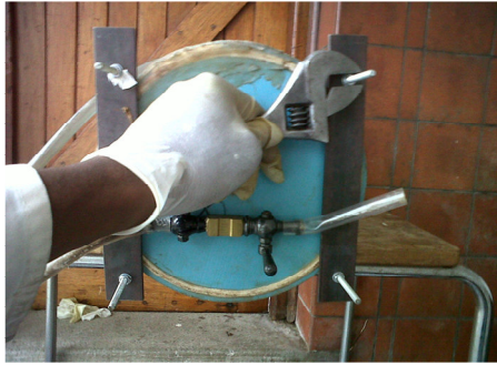
a) Undoing the rods tightening the lysimeter plates
