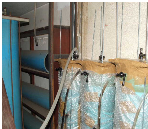
Figure 3.9 shows a plastic tube supplying water into the lysimeter.
