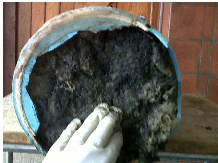
d) Removal of sand layer for drainage at the base of the lysimeter
