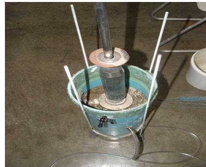
Figure 3.6: Marshall Compaction hammer resting on compacted waste.
