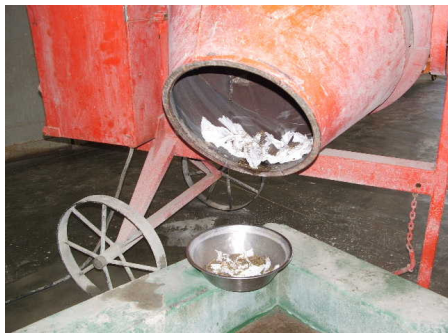
Figure 3.5: Mixing of the refuse using a concrete mixer.
