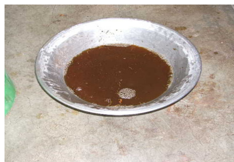
Figure 3.4: Water accumulated in a gathering pan after 24 hrs.
