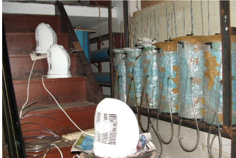
Figure 3.2: Layout of fan-heaters and bubble-wrapped lysimeters.
