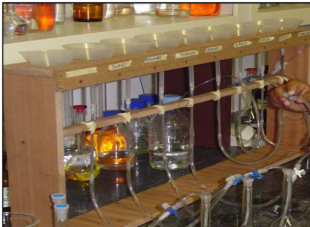
Figure 4.9: The nitrate cadmium reduction columns assembled in the laboratory by the author of this report ( Author ).
