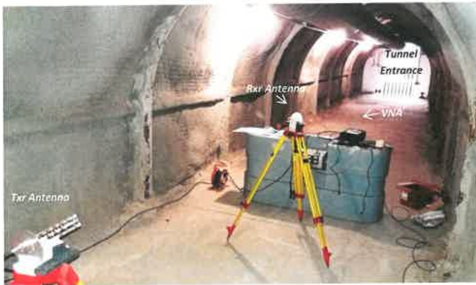
Figure 6.1 Wideband Measurement Test Setup in WITS mock-tunnel
