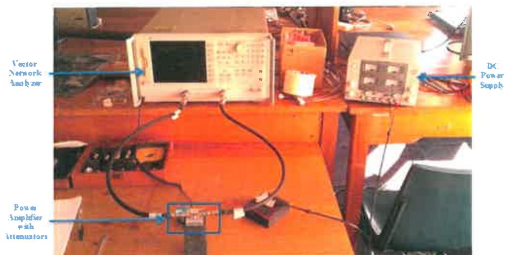
Figure H1 Calibration test setup for HGA
