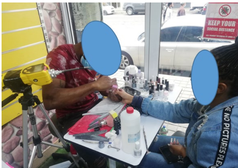
Figure 2.4 Task based exposure assessment using a photoionization detector during a nail application process
