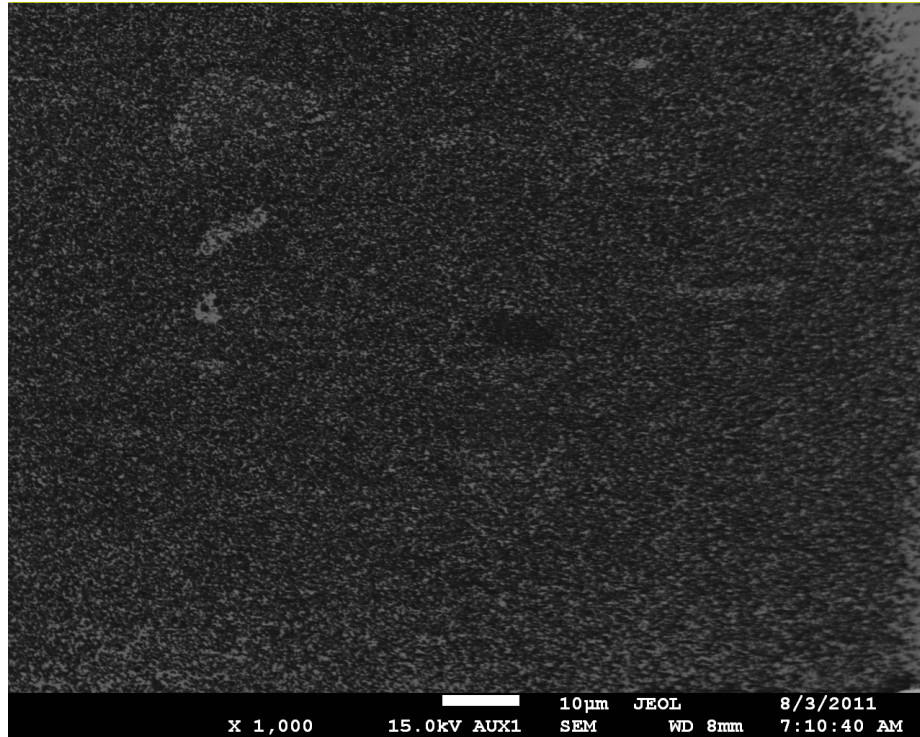
Figure 4.23: SEM showing light and dark spots in the diamond table of the 2μm powder pressed standard.
