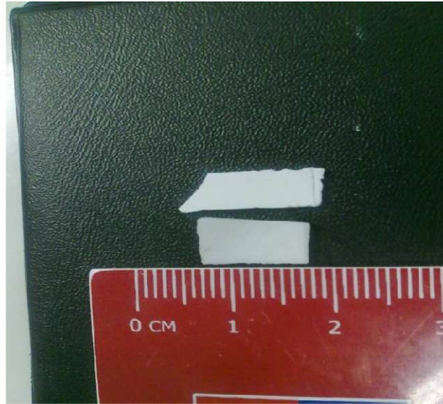
Figure 4.8: Photograph showing Sample 42 prepared using a 10% (w/v) alumina suspended in isopropanol at pH 3.7, 32.5V/cm for 1 hour.
