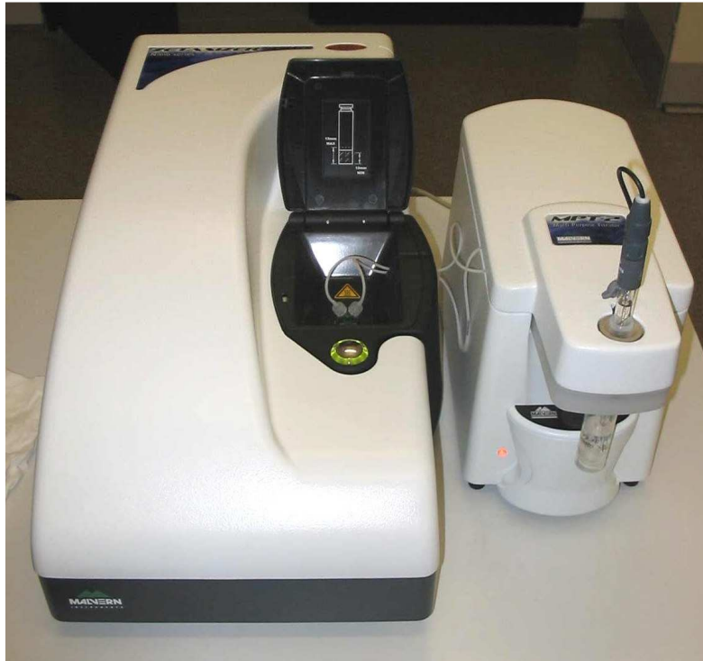
Figure 3.7: A picture of the Malvern Nanosizer with the auto-titrator and pH meter on the right.
