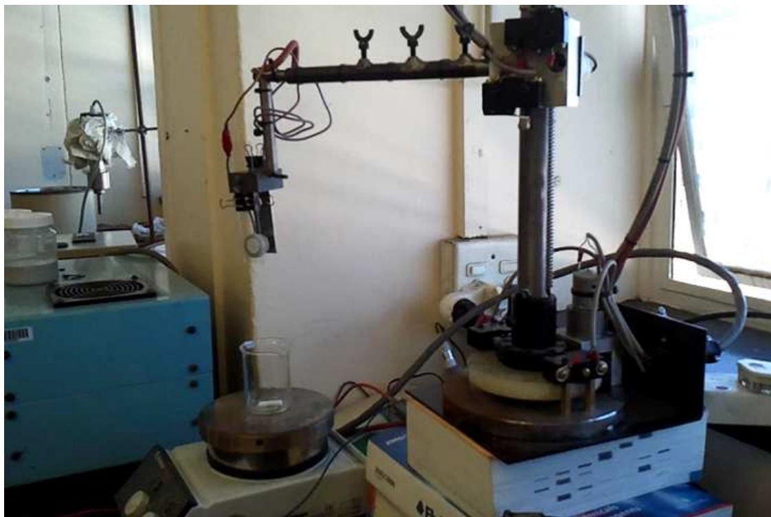
Figure 3.5: Robotic arm to automate movement of electrodes between two different suspensions for laminate deposits.
