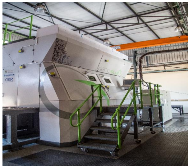
Figure 3.3: Aeroswift™ 3D printing machine available at CSIR, Pretoria.
