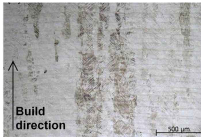
Figure 1.2: Microstructure of SLM produced Ti6Al4V (Vrancken et al. , 2012).
