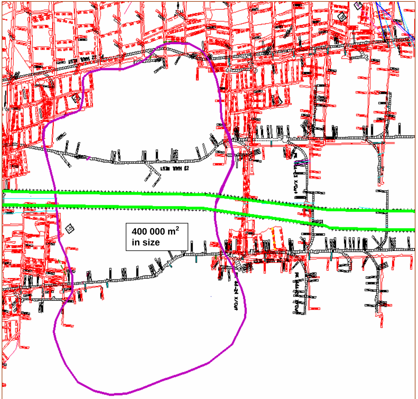
Figure 2.4 A plan view of a pothole intersection on the Merensky horizon (Novy 2006: 8)
