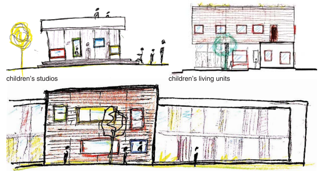
figure 141: Sketches showing how materials that were used in children's living units were reinterpreted to create an architectural language for each project component.
