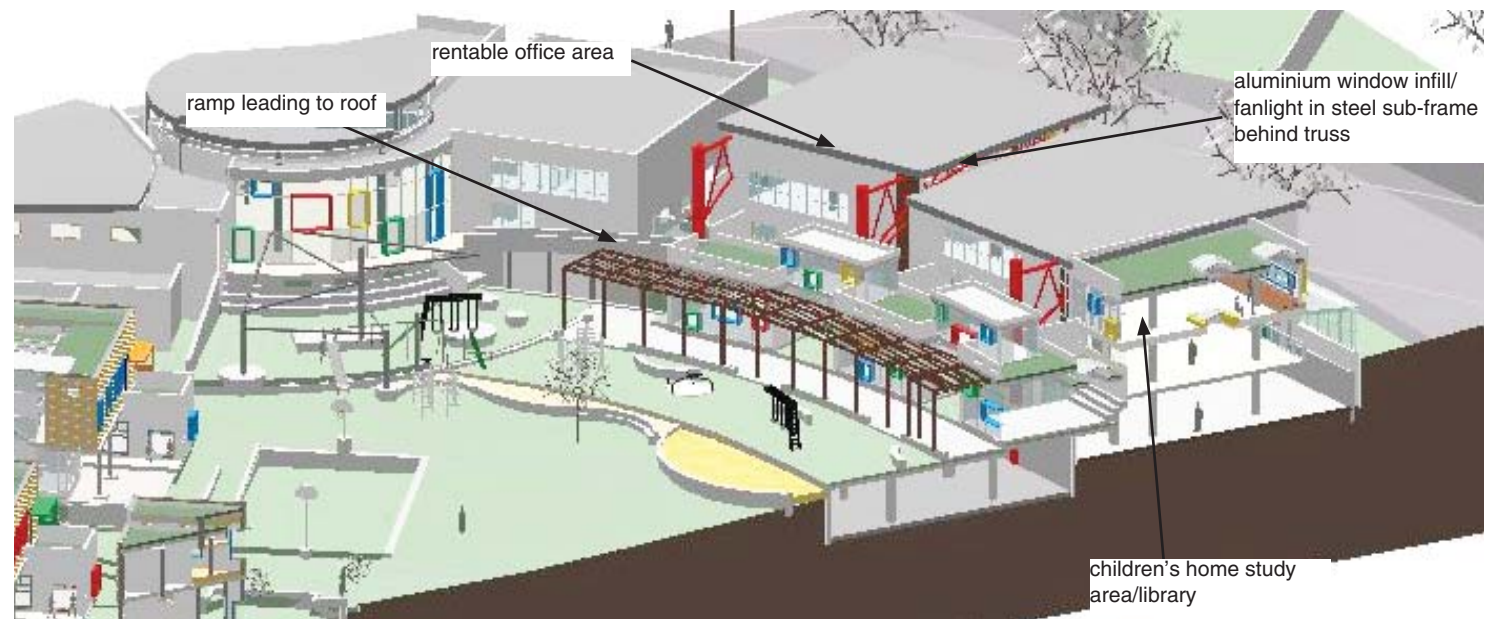
detail 3: axonometric/concept models of truss system (highlighted in red)
