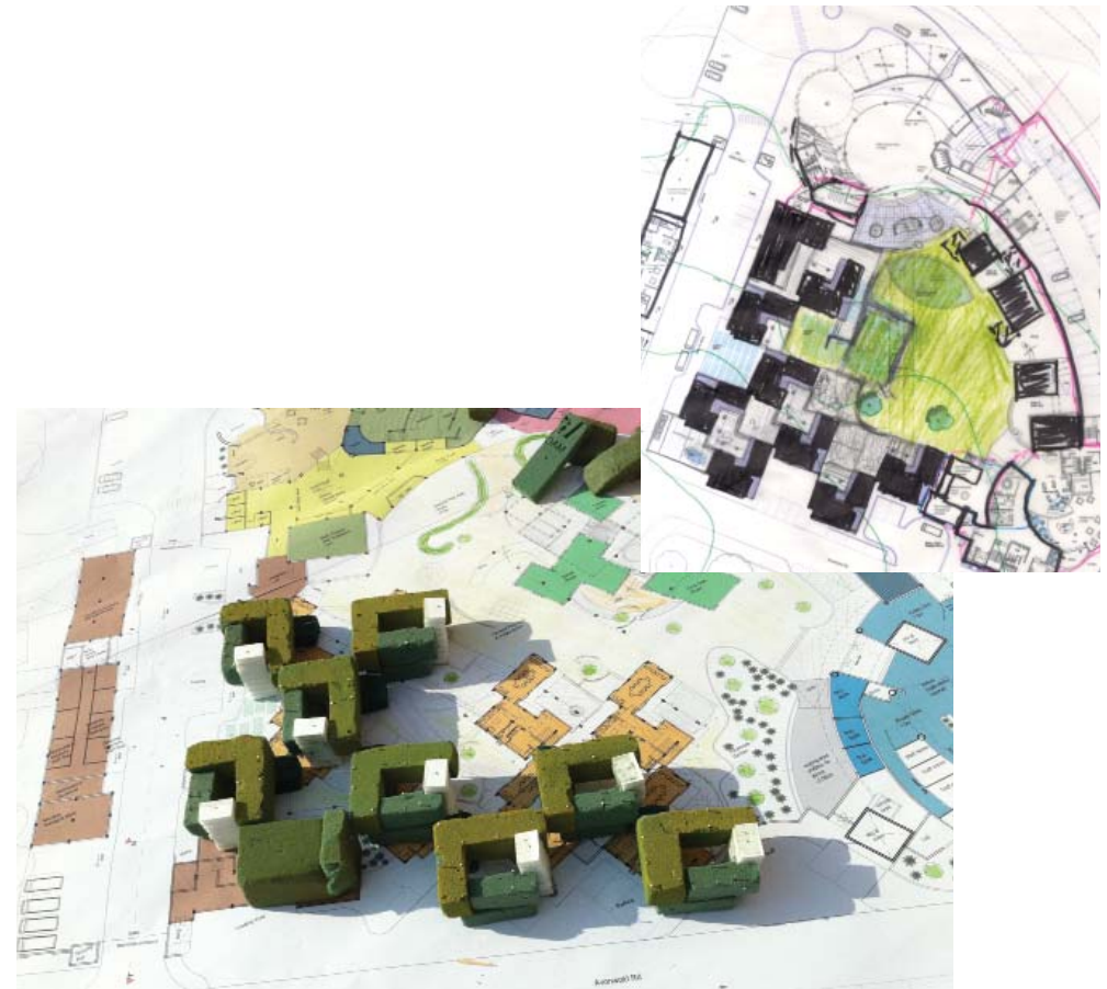
figure 131: Design methodology: switching between drawings and models.
