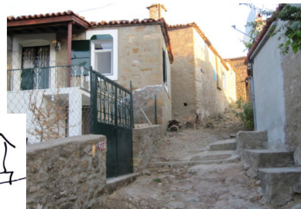
figure 42e: The social organisation layout of this village was all a response to different methods involving site location – using the site for control and protection (view), sun advantages, etc. Houses were built close together and were staggered to break strong winds. Natural resources were available to construct and sustain the houses. Houses were built along contours and the various levels also provided visual interaction. The village's growth would only be limited by the site's natural condition.
