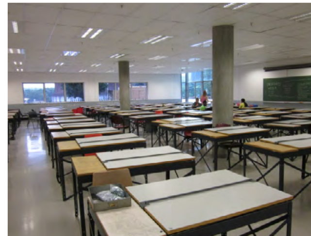
Figure 72: The rectangular shape of a UA studio, with windows on the short side, results in poor natural lighting, insufficient ventilation, and thermal discomfort. (Author, 07.02.2012).
