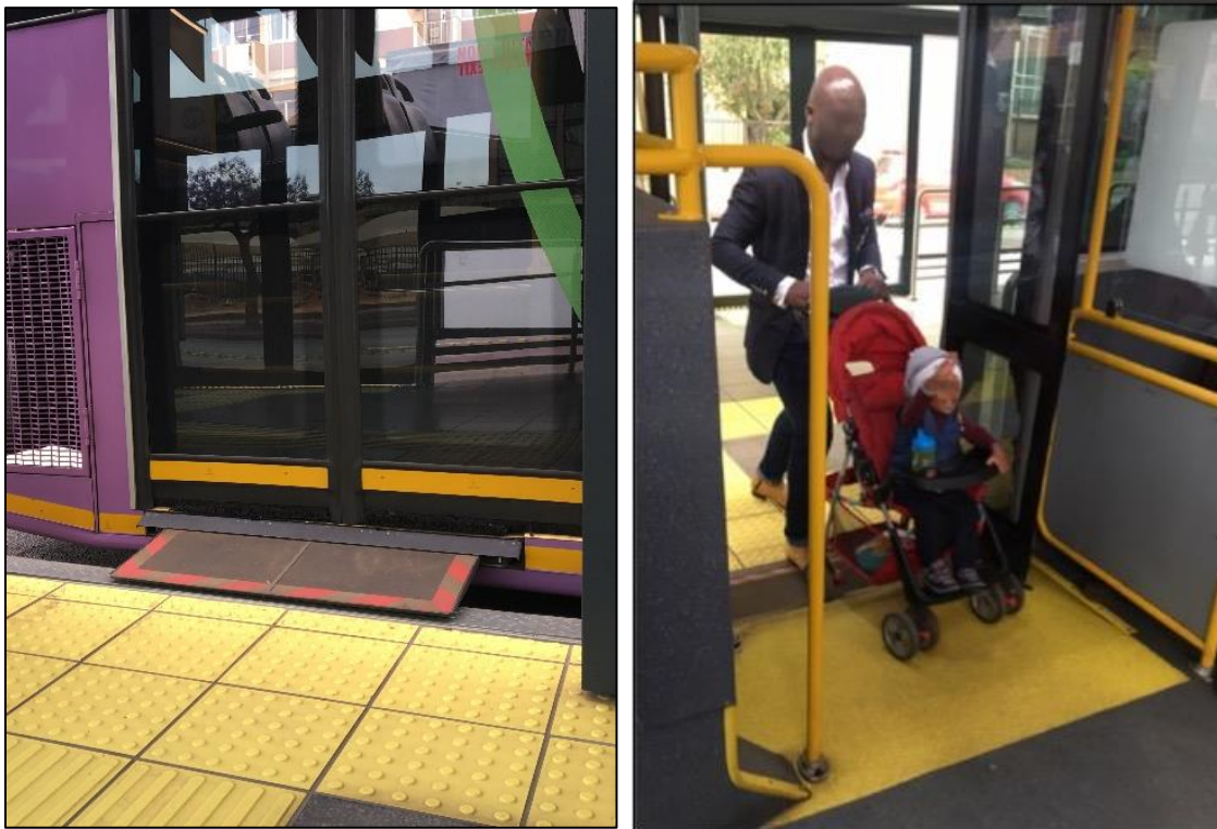
Figure 11: Ramp on the BRT platform
