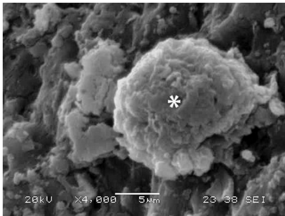
Figure C.7 A foreign particle (asterix) on the surface of the skin (sample 5-3). The particle showed a high calcium count when analysed with EDS
