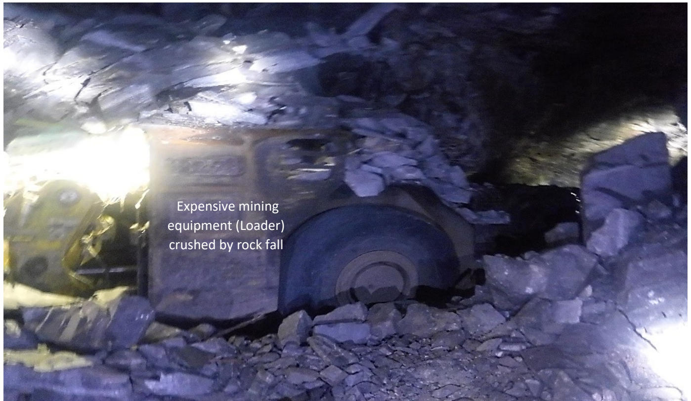
Figure 8-4: Picture of an underground mine accident that involved fall of ground (rock fall) in weak zones attributed to geological structures.
