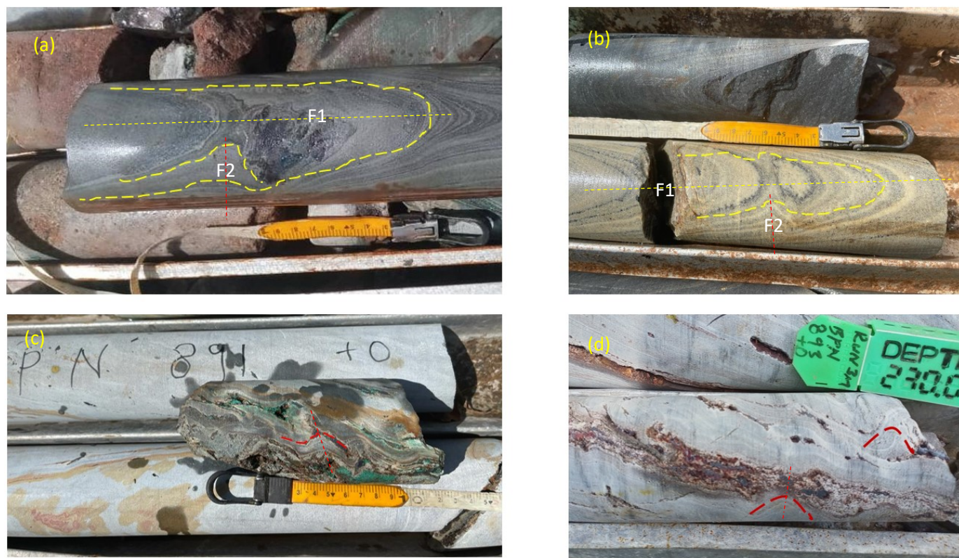
Figure 6-9: Folds observed in core logged. (a) Ore shale with well moderately open parasitic fold. Two generations of folds are observed here. F1 fold is refolded in folding event F2. (b) Folding observed in ore Hangingwall quartzite. (c) Folds in highly weathered ore shale unit with malachite mineralization (d) moderately open to tight folds developed in ore shale unit with chalcocite mineralization.
