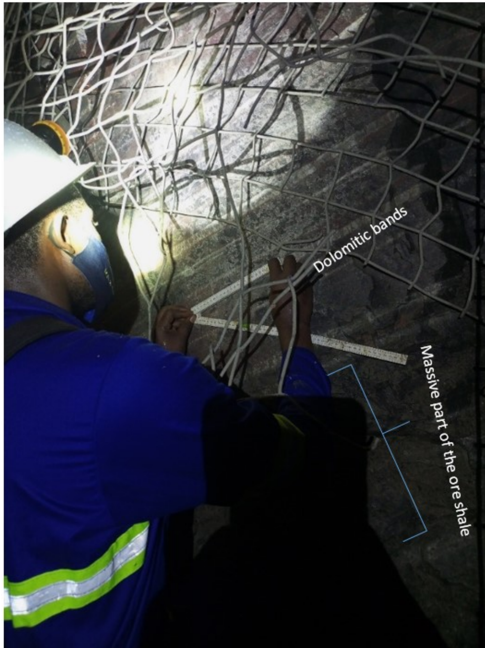
Figure 4-7: Underground picture from 2400mW showing distinct bedding in the Ore shale Unit.
