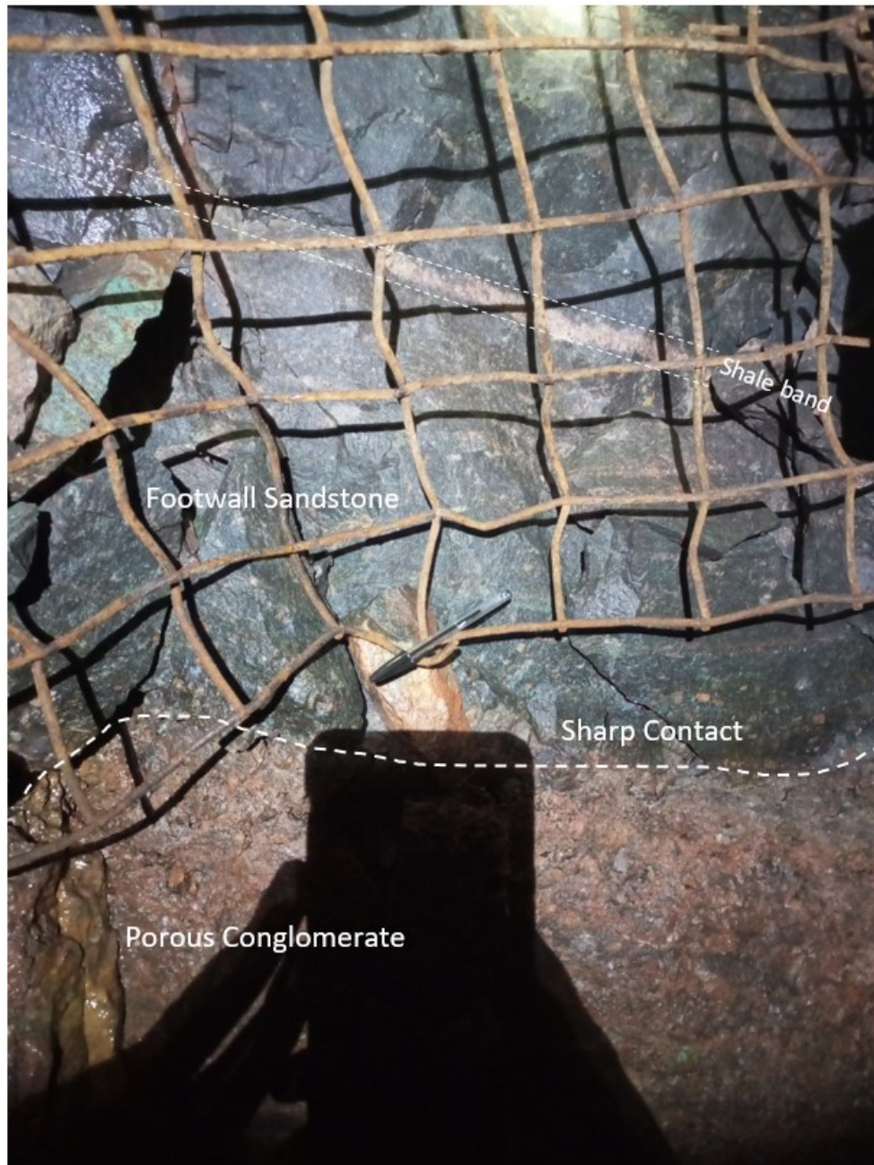
Figure 4-5: Underground picture showing the contact between the Porous Conglomerate and the Footwall Sandstone. Note pen for scale. Picture taken on 780 mL, 2400 MW crosscut (Figure 1-3).
