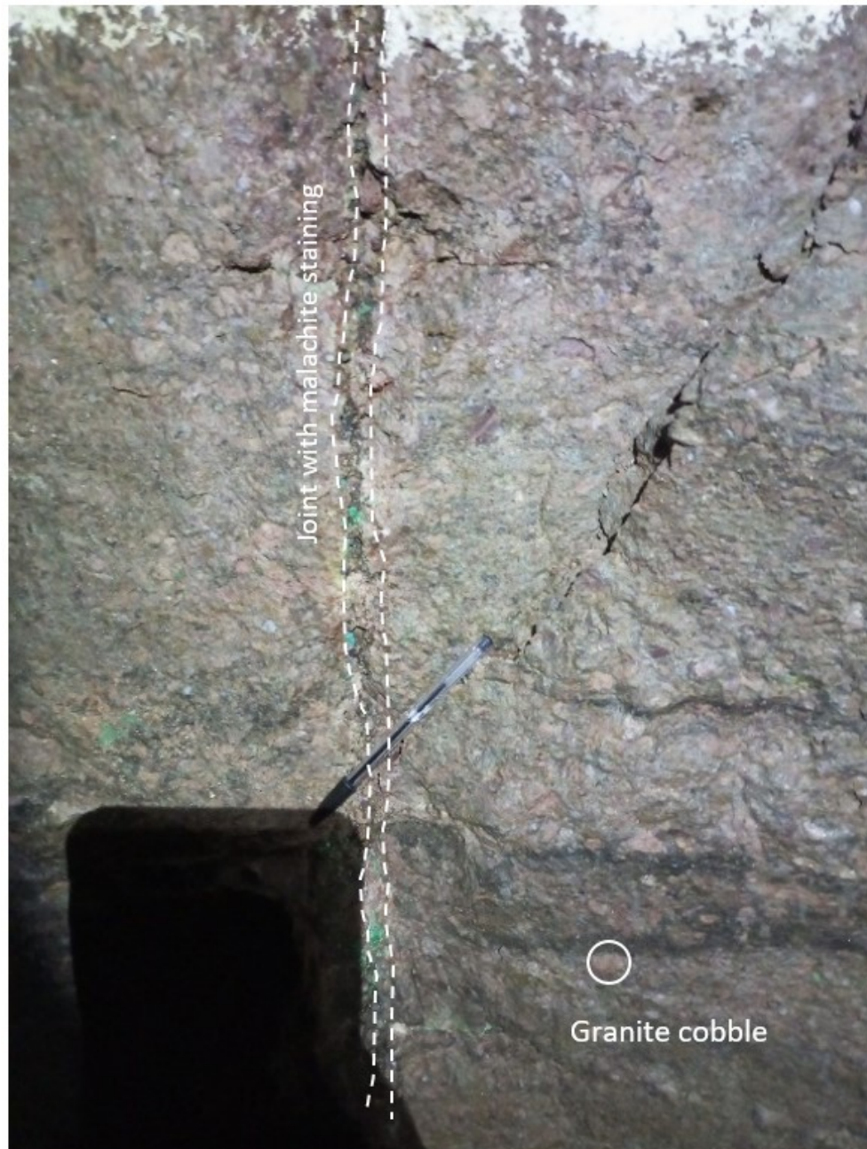
Figure 4-4: Underground picture taken from 2400mW crosscut facing east showing the Porous Conglomerate with malachite staining along the joints.
