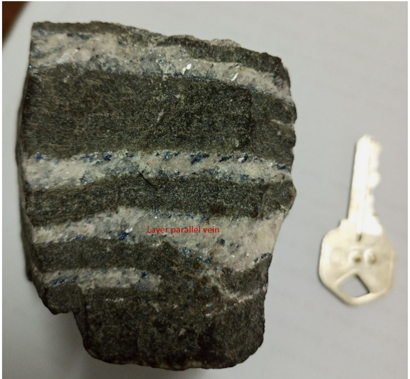
Figure 4-8: Hand specimen of the Ore Shale Unit showing bornite mineralization occurring in layer parallel veins
