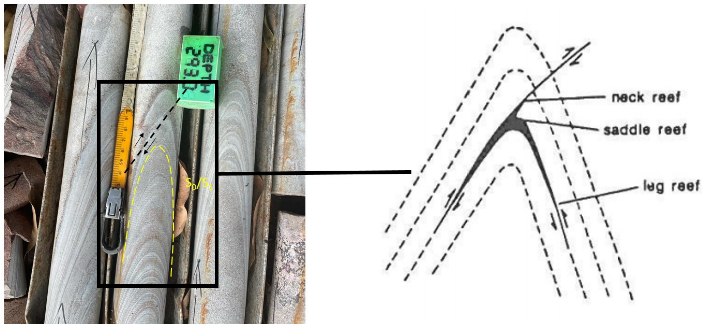
Figure 6-19: Core photo from BPN 881 showing bedding discordant fault resulting from flexural slip on one limb that goes through and breaks across the fold hinge. Schematic illustration done after (Cox et al., 1991)
