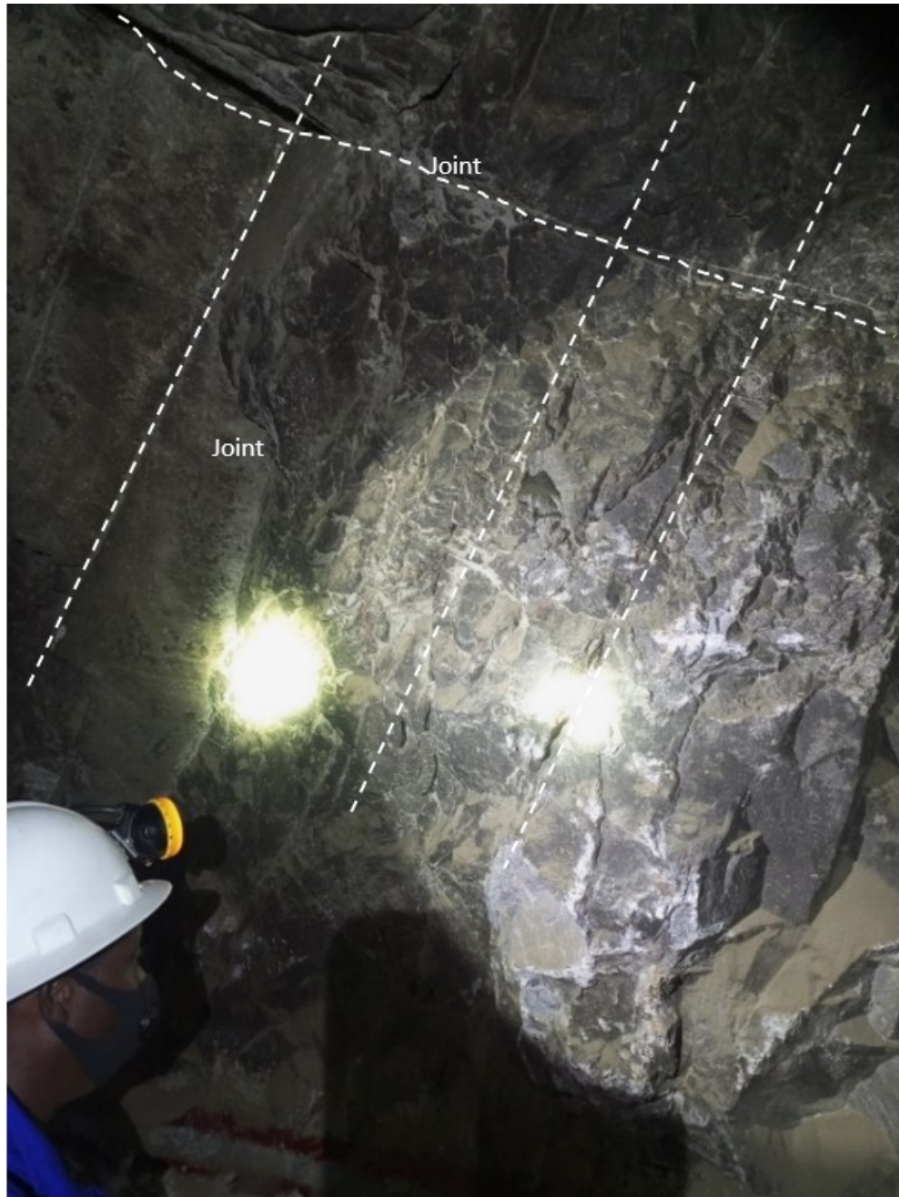
Figure 4-2: Underground picture showing massive and jointed Footwall Quartzite.
