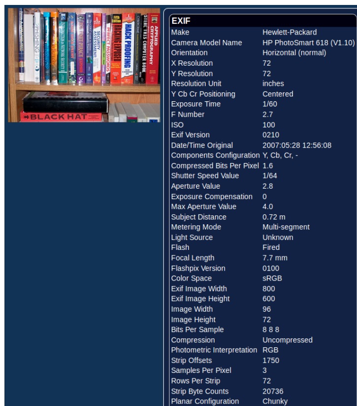
Figure 2.5: The figure show us the camera's make and camera model name (HP PhotoSmart 618), and also the original time this photo was taken 28-May-2007 [7].
