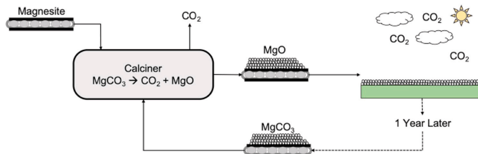
Fig. 10. Schematic of potential use of mine tailings to capture carbon dioxide from the atmosphere [19].
