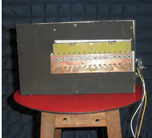
(a) The transmitter and receiver arrays mounted on the front of the box.
