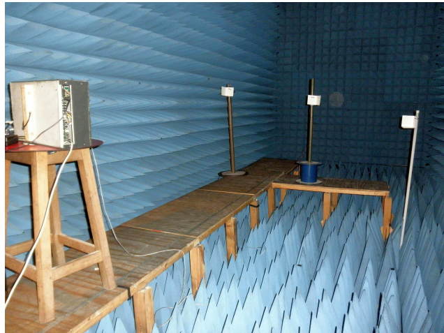
(a) A target detection experiment in the anechoic chamber with three targets.
