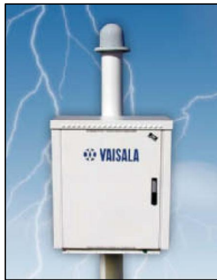
Figure 21: Vaisala LS700 Cloud-Ground Lightning Sensor (Bardo 2005).
