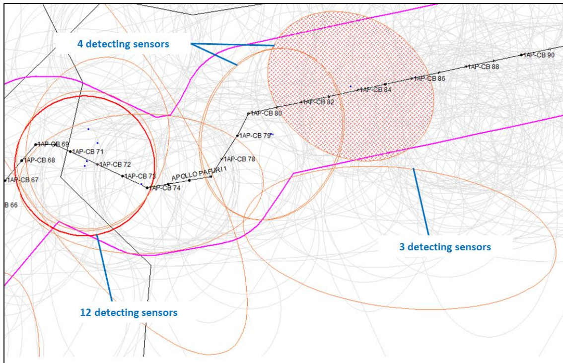
Figure 29: Confidence ellipses for individual strokes detected by twelve, four and three sensors 21 .
