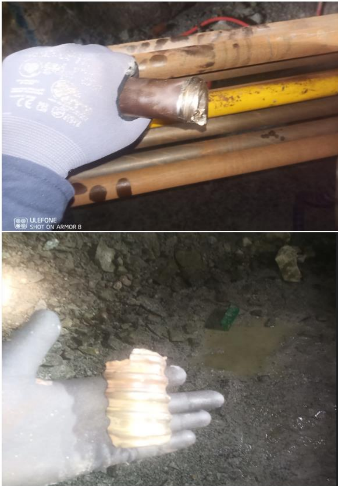
Figure 4-28: Broken drill bit shanks
