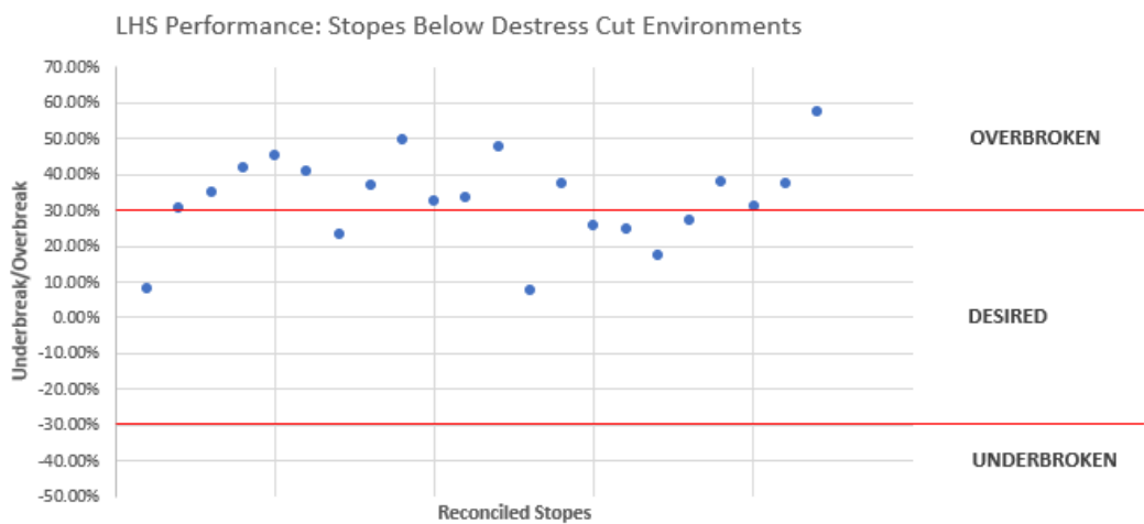
Figure 4-7: Stopes below de-stress cut environments
