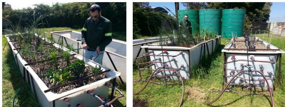
Figure 3-1: The experimental constructed wetlands at the IMWaRU site, Wits University showing the five zones of vegetation (left), the planted and unplanted wetlands side-by-side and the JoJo tank set-up (right). The outlet configurations (inlet configurations are not shown but are of the same design), the syphon break and the sample ports are also visible (right).
