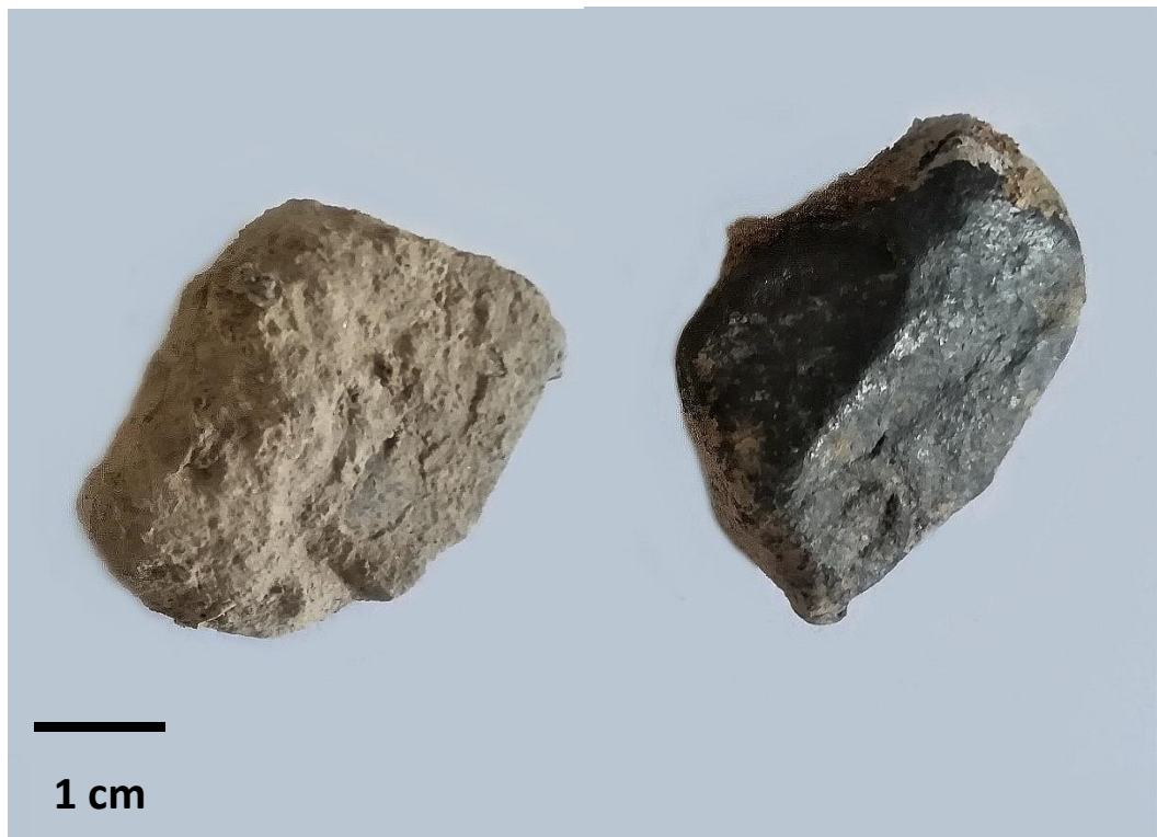
Figure 3.1. Piece OBP-3653-1, recovered from YRS dec. 8, before (left) and after (right) acid cleaning.
