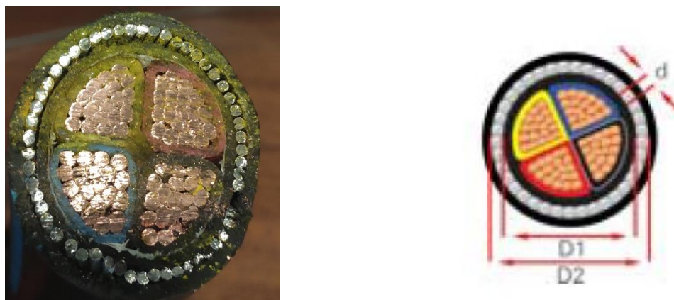
Figure 3.13: Sample cross-section of 95mm 2 cable and dimensions
